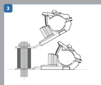
Add a spacer between Ratchet P Clamps to speed installation and maintenance of stacked wire bundles.
