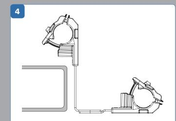
90° angle mounting plates enable you to work around obstacles and protect wire from contacting moving parts.
