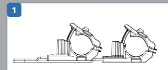
You can piggy-back Ratchet P Clamps by using different length mounting plates to secure parallel cable configurations.
